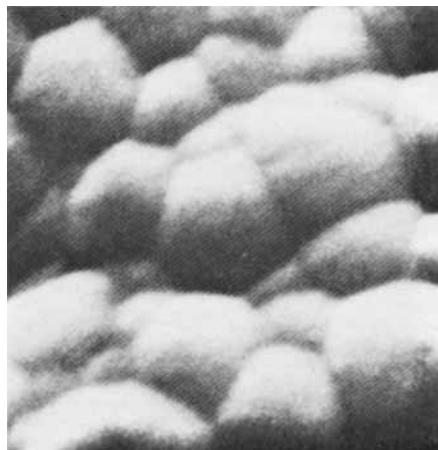
Fig. 7. SEM micrograph of plasma-formed polyethylene. Power level 5 W, partial pressure 20 microns (49,000 \times ).
