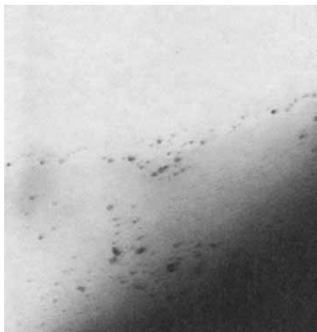
Fig. 4. TEM micrograph of plasma-formed polyethylene. Power level 5 W, partial pressure 20 microns (77,000 \times ).
